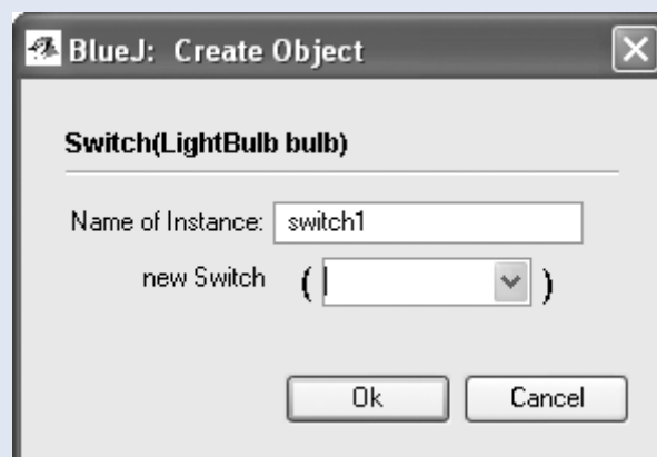
Figure 17 The Create Object dialogue box that appears when a new instance of Switch is created, requesting the name of an instance of LightBulb that will be passed to the Switch constructor
